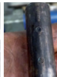
Fig. 5. Spray pipe when dismantling the pipeline
