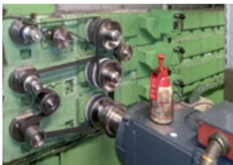
Fig. 6. Belt drive after reconditioning.
