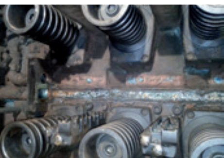
Fig. 1. Drawing area of a MMH after 65,000 hours of operation.
