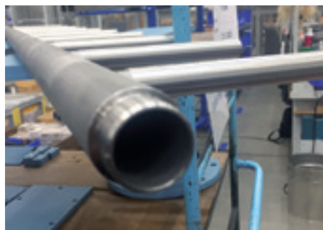
Fig. 7. New spray pipe.
